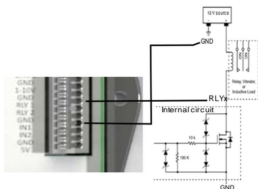
Figure 4: Wiring external relays
