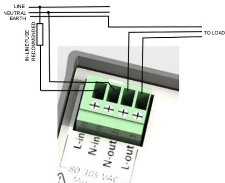
Figure 3: Wiring for external AC Loads
