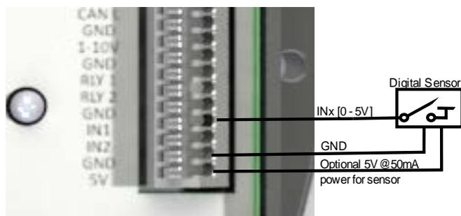
Figure 6: Wiring for digital inputs
