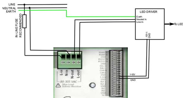
Figure 5: LED drive with 1-10V dimming
